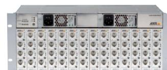
When AXIS Q7414 blades are used with AXIS Q7900 Rack, up to 56 analog cameras and audio channels can be supported in one 4U, 19-inch rack.
